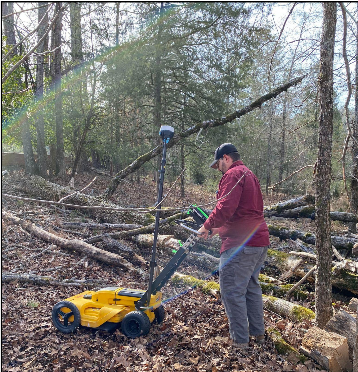
Figure 3: Sean McConnell, PhD operates a Leica DS2000 dual channel GPR at Penfield.
